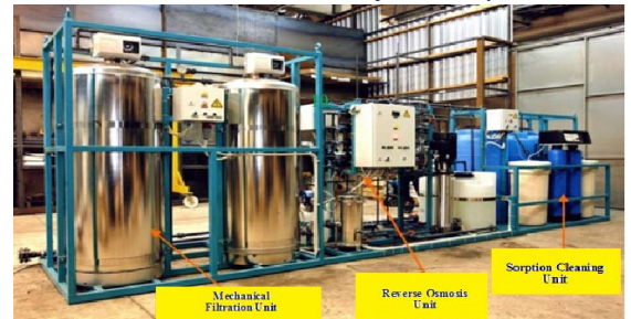
Modular LRW treatment complex
